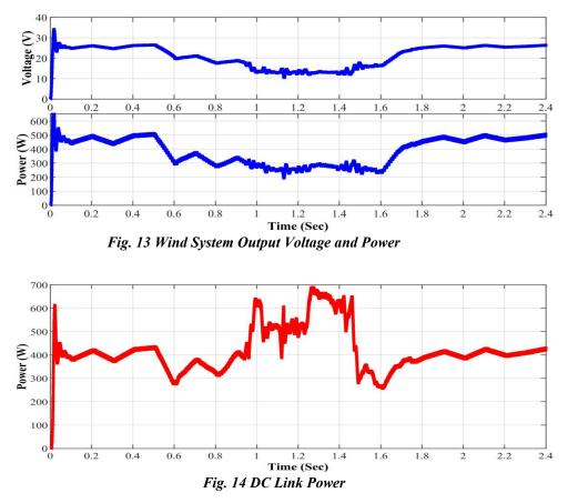
The Fig. 14 shows the DC link power of hybrid system under real-time solar irradiation and wind speed data.
