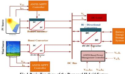
Fig.1 Basic Topology of the Proposed Hybrid System
