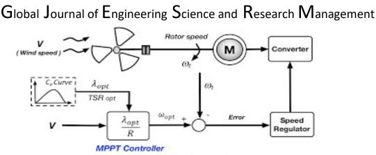
Fig. 7 Tip speed Ratio control
