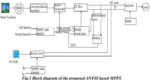
Fig.3 Block diagram of the proposed ANFIS based MPP1.
