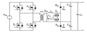
Fig. 9. Isolated Bidirectional DC-DC Converter
